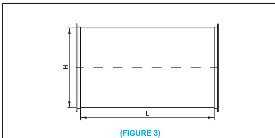
The baffles are filled with non-inflammable sound absorbing material , erosion and hygroscopic protected and allowing velocities up to 20 m.p.s.
